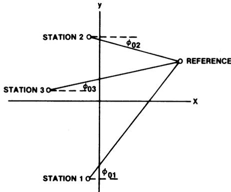
Fig. 6. Angle definitions for reference and three stations.
