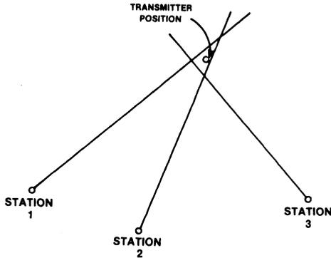
Fig. 10. Bearing lines from three direction-finding systems.
